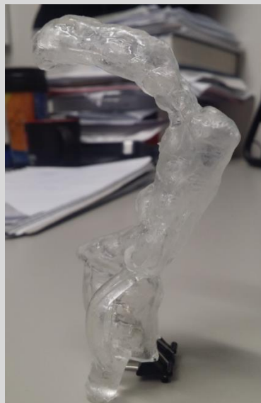
Figure from ongoing research: Inverse Casted Upper Airway Model Sample (from 3D Printed Mold). Reconstructed from axial MRI images, includes mouth, oro and laryngopharynx, epiglottis up to upstream of first airway bifurcation
